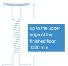
C-PE support 38 x 38 x 1 mm with 4 cams
