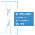
C-PE support 38 x 38 x 1 mm with 4 cams
